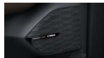
Rear door Coaxial 2way speaker
