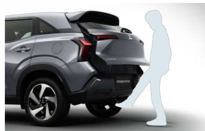
Hands-free power tailgate Open and close easily by put foot under rear bumper.
