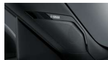
Front dome tweeter on A pillar
